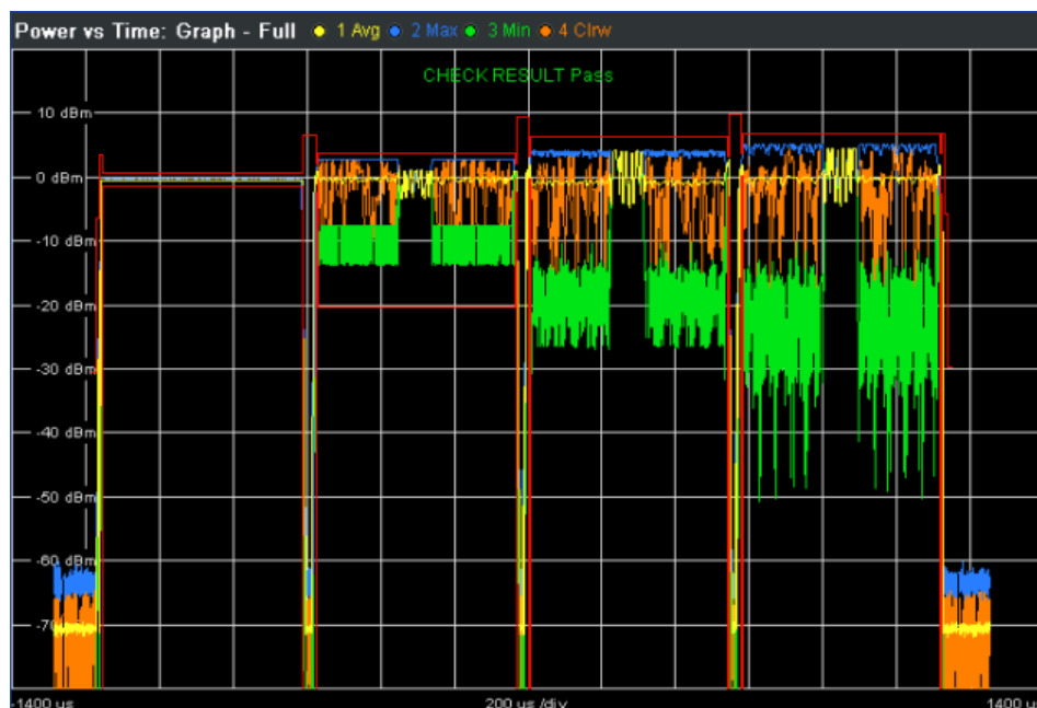
Fig. 3-10: Full Burst view in Power vs Time
